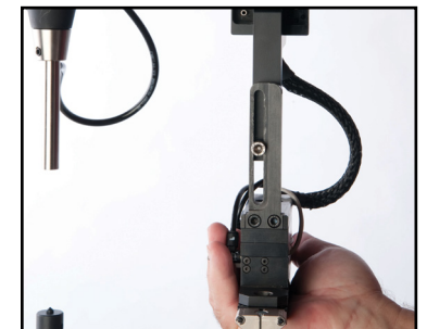
New T-bracket and shuttle with integrated connectors.
