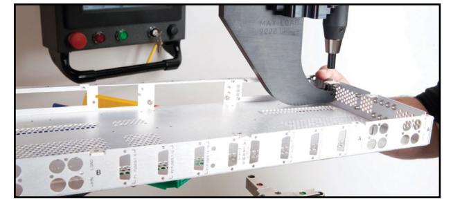
Manual J-Frame in combination with 24” (610mm) throat depth.
